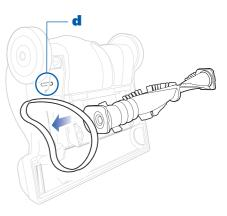
With the Brush Roll free, inspect for any hair build-up or string; if present, carefully cut out with scissors; take care not to damage the bristles.
